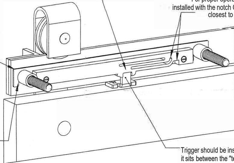
Trigger should be installed so that it sits between the "teeth" of the catch on the device.
