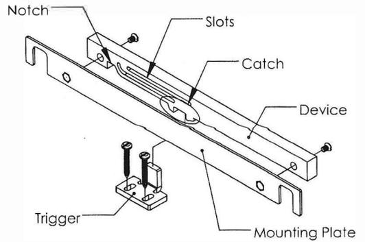
NOTE: Instructions apply to all standard 11 inch and 17 inch Soft Stop systems. Mounting plates with custom hole patterns greater than 11 inches can be manufactured upon request.
