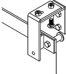
Using the provided hex head bolt attach the second track to the extender bracket as shown.
