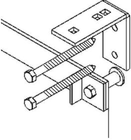
Using the provided 3/4" carriage bolts and keps nuts, attach the bypass extender brackets to the wall brackets as shown.
