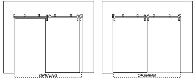
Where doors slide freely, in either direction and stack within the opening to leave only one side of the opening clear.
