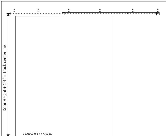
Use the front track to determine the spacing for the bypass bracket pilot holes.
