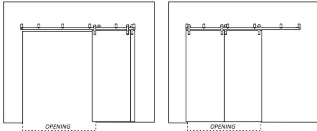
Where doors stack collectively on either or both sides of the opening to leave the opening clear and free from obstruction.
