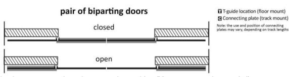
2 barn door hardware sets, 2 tracks each = 2× one door width -½" (no connecting plate needed)
