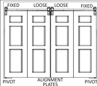
Installation of a 4-door configuration is nearly the same as installing two 2-door hardware sets end-to-end, with the fixed hangers on the two outer door panels and the rolling hangers on the two middle door panels.
