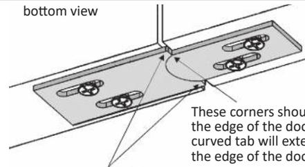
These corners should align with the edge of the door panel. The curved tab will extend beyond the edge of the door panel by 1/4".
