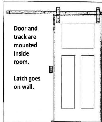
When the door and track are mounted to the wall on the inside of the room, the dust box and latch mount in the wall, and the strike plate mounts on the edge of the door.
