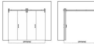
The stacked doors will hang over into the opening up to 4" in the fully opened position, with a minimum wall overlap of 1" on each side when fully closed.
