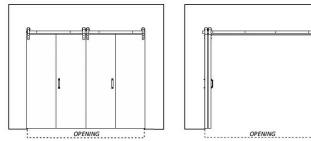
The stacked doors will hang over into the opening up to 4" in the fully opened position, with a minimum wall overlap of 1" on each side when fully closed.
