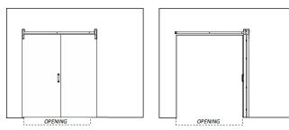
The stacked doors will not hang over into the opening in the fully opened position, with a minimum wall overlap of 5" on the stacking side and 1" on the closing side.
