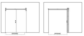
The stacked doors will not hang over into the opening in the fully opened position, with a minimum wall overlap of  $5^{\prime\prime}$  on the stacking side and  $\,1^{\prime\prime}$  on the closing side.
