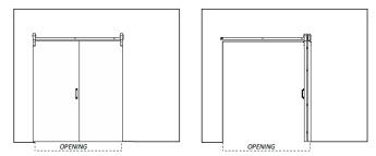
The stacked doors will hang over into the opening up to 4" in the fully opened position, with a minimum wall overlap of 1" on each side when fully closed.
