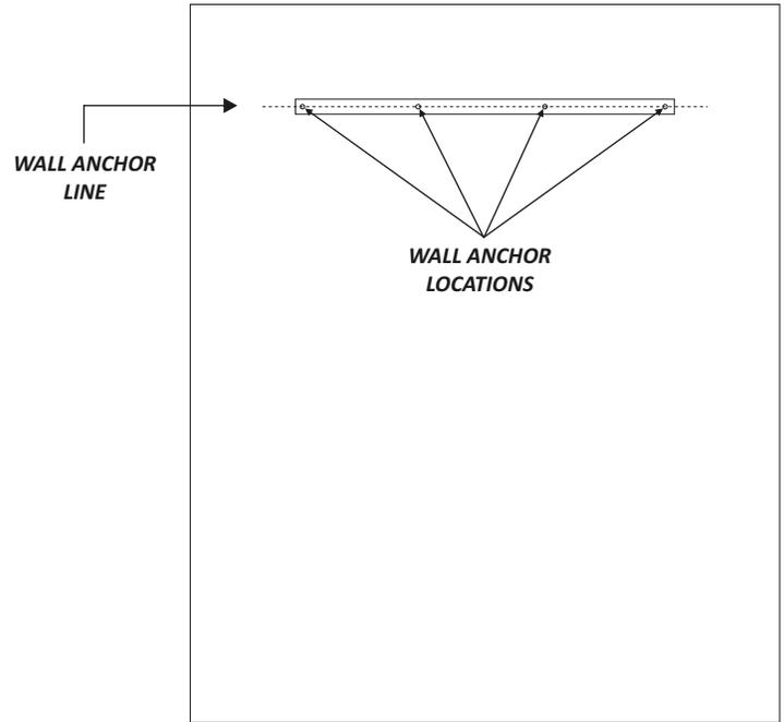
Using the provided drywall screws, attach each track wall bracket as shown.
