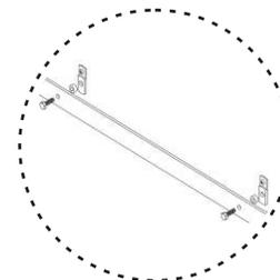
Use the remaining hex lag bolts and spacers to finish attaching the track at the remaining connecting points.
