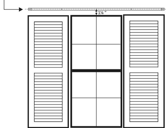
**Note:** The track should be installed a minimum of 1 1/8" above the window to ensure the roller has clearance.
