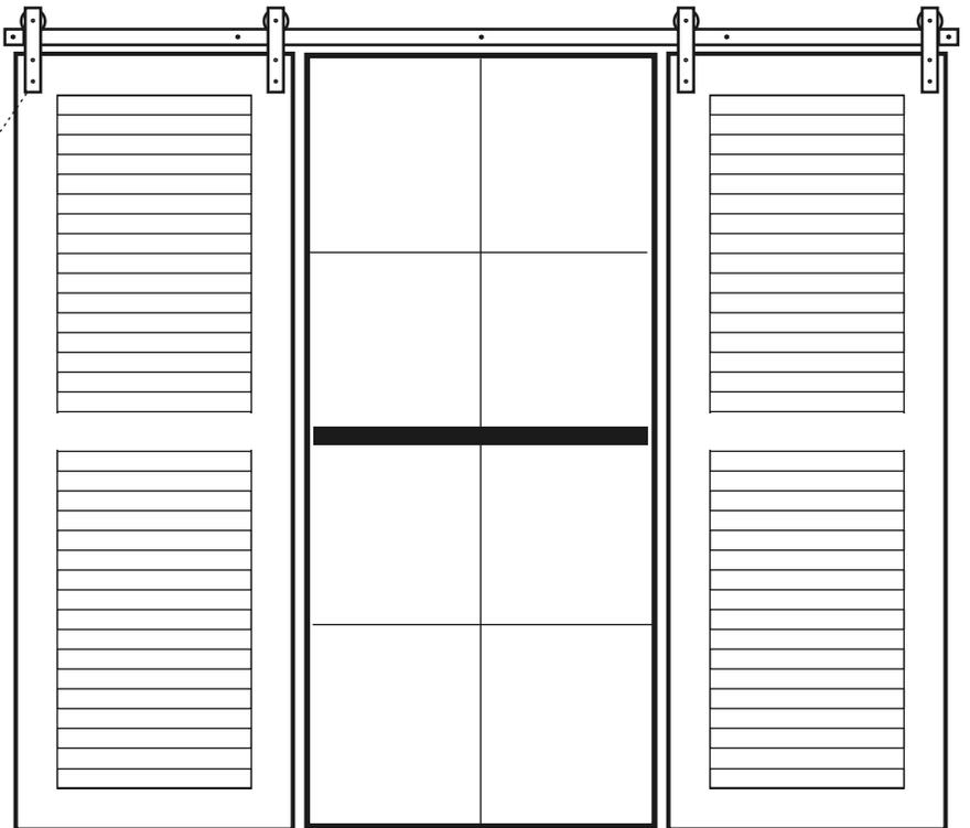
Once the 1/4" hex head lag bolts are through the item, hang the shutter from the track in your desired position and continue to install the lag bolt so it goes into the wall.
