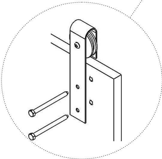
To install the hanger, insert the provided 1/4" hex head lag bolts through the hanger on the front of the item as shown.
