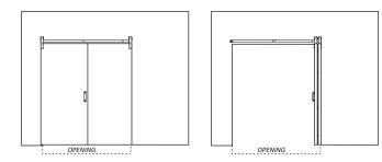
Door will hang over into opening up to 4" when in an open position [min. 1" overlap on both sides]
