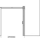
Door will hang over into opening up to 4" when in an open position [min. 1" overlap on both sides]
