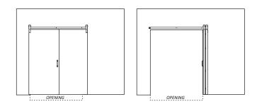
Door will NOT hang over into opening, allowing for a completely **clear opening** *[min. 1" overlap on closing side and 5" overlap on stacking side]*
