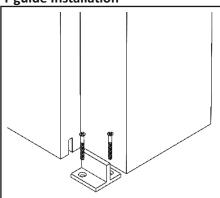
Using the T-guide screws, attach the T-guide to the floor by aligning the edge of the guide with the edge of finished opening as shown above.
