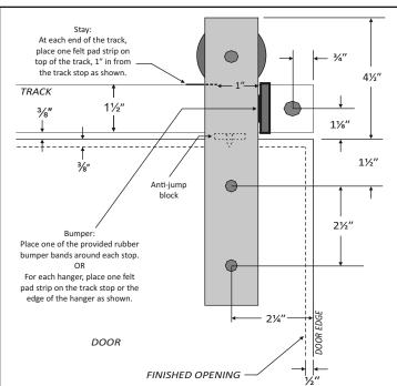
In the closed position, the door should overlap the wall a minimum of %" at the top and a minimum of ½" on both sides.
