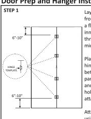
Lay both panels front side down on a flat surface with inner edges flush through the middle and on top.
