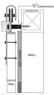
Standard hardware set + 1/2" extension kit installed where casing, base, or other trim is up to ½" thick.
