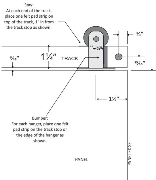
In the closed position, the door should overlap the wall a minimum of 3/8" at the top and a minimum of 1/2" on both sides.
