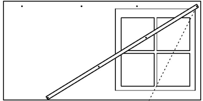
Using a hex lag bolt, track stop, spacer and washer, connect one end of the track to the wall using the pre-drilled hole closest to the opening as shown in the diagram.
