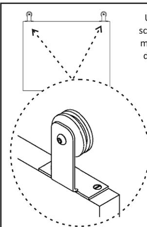
Using the top mount screws, attach the top mount hangers to the door as shown in the diagram.
