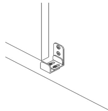
Using the adjustable guide screws, attach the adjustable guide to the wall by aligning the edge of the guide with the edge of the finished opening as shown above.
