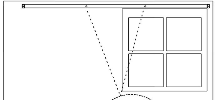
Using the remaining hex lag bolts, spacers and washers finish attaching the track at the remaining connecting points.
