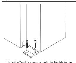
Using the T-guide screws, attach the T-guide to the floor by aligning the edge of the guide with the edge of the finished opening as shown above.
